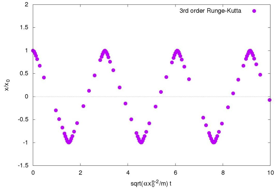
AHO:  $V(x) = \alpha x^n$ ,  $n = 20$ ,  $\alpha = 1.0$ , ABS  $x(t=0) = x_0$ ,  $v(t=0) = 0$ ,  $\delta_{\text{abs,max}} = 0.001$ ,  $\tau_{\text{initial}} = 1.0$
