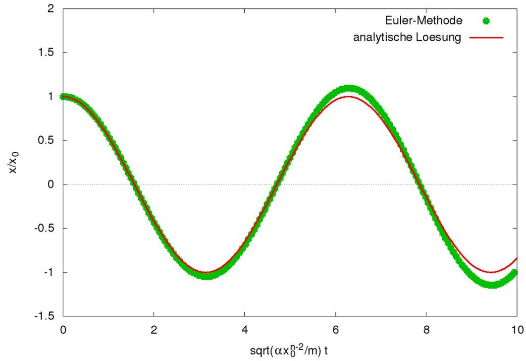
AHO:  $V(x) = \alpha x^n$ ,  $n = 2$ ,  $\alpha = 0.5$ , ABs  $x(t=0) = x_0$ ,  $v(t=0) = 0$ ,  $\delta_{\text{abs,max}} = 0.001$ ,  $\tau_{\text{initial}} = 1.0$
