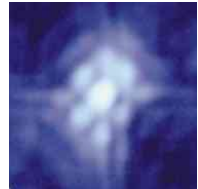
LDOS and conductance map: Zn impurity in BiSCCO at V=-1.5 mV
