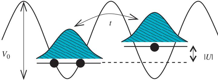
Figure 1. Cold atoms in an optical lattice of strength  $V_0$ , shown here with hopping  $t$  and negative onsite interaction  $U$ . This situation corresponds to an attractive Hubbard model where multiple occupancy of lattice sites is energetically favorable.
