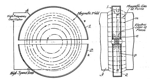
The apparatus consists of two D-shaped electrodes (called simply D's by accelerator physicists). They are connected to a radio-frequency (RF) voltage of frequency f. The voltage at the electrodes is thus changing with time by
