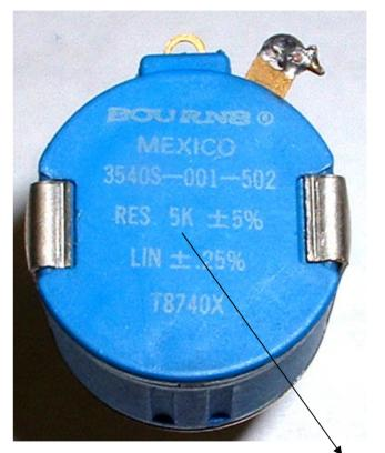
Measuring resistance across tabs 1 and 3 should yield the full resistance  $(5k\Omega)$ . Measuring the resistance between tabs 1 and 2 will yield the resistance between tab 1 and the wiper connected to tab 2.
