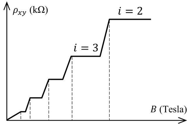
**Abbildung 2.5:** Schematic representation of the measured Hall resistance.
