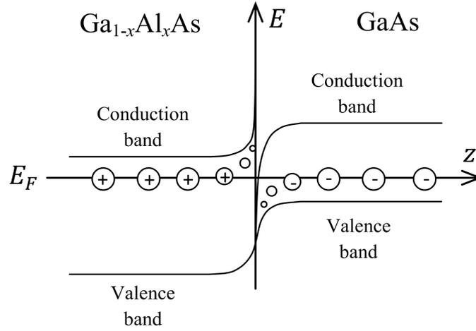
**Abbildung 2.4:** The scheme of the energy bands of the  $\text{Ga}_{1-x}\text{Al}_x\text{As}/\text{GaAs}$  heterostructure. The charge density of the system is  $\sim 10^{11} \text{ cm}^{-2}$ .
