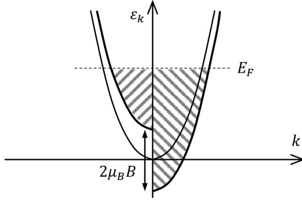
**Abbildung 2.2:** Energy spectrum of the conduction electrons in an external magnetic field.
